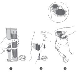
Install the roller brushbar onto the floor brush, and turn the roller brushbar lock to the locked position. Then reinstall the roller brushbar cover.
